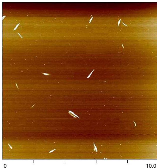
Fig. 1. The AFM imaging of ramie nanocrystallites from a dilute suspension (scale bar = 2 μm).
